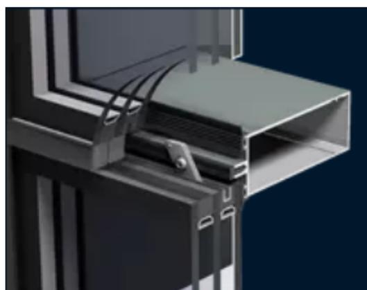
CONCEPTWALL 50 AVEC VITRAGE CLAMÉ STRUCTURELLEMENT OFFRE UNE SURFACE VITRÉE CONTINUE DONT LES VITRAGES SONT CLAMÉS MÉCANIQUEMENT PAR DES SERREURS. LE JOINT ENTRE LES FEUILLES DE VERRE PEUT ÊTRE FINI PAR UN JOINT DE SILICONE OU UN JOINT EPDM. EN RAISON DE L'ABSENCE DE PROFILÉS DE RECOUVREMENT TRADITIONNELS À L'EXTÉRIEUR, LE VITRAGE CLAMÉ STRUCTURELLEMENT OFFRE MOINS D'OBSTACLES VISUELS POUR UNE CONCEPTION MINIMALISTE DU MUR-RIDEAU.
